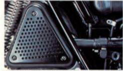
Silent-type muffler minimizes noise for city cycling and is neatly cradled over rear tire.
