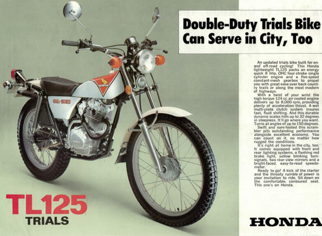
An updated trials bike built for onand off-road cycling! This Honda lightweight TL125 packs an energy quick 8 hhp, OHC four-stroke single cylinder engine and a five-speed constant-mesh gearbox to propel you with great ease over back country trails or along the most modern
